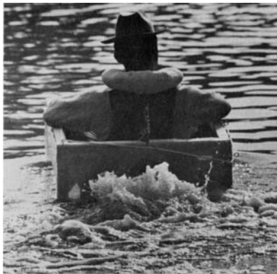
The design limitations disallowed gasoline engines. This student used an auto starter with a battery as his propulsion. He is sailing along here at 6 m.p.h.
