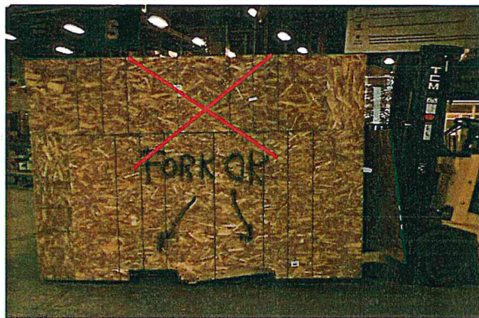
INCORRECTLY CRATED SHIPMENT
