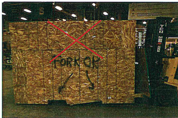
INCORRECTLY CRATED SHIPMENT
